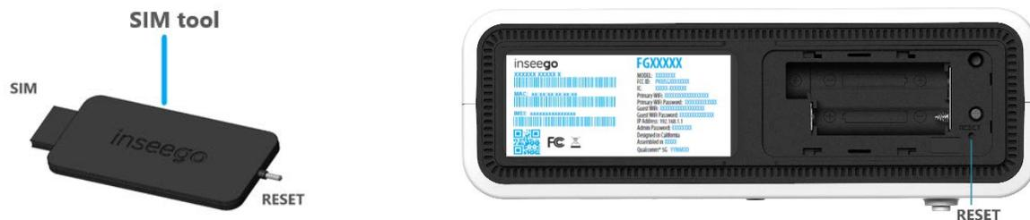
3. Press the SIM tool on the button for about five to six seconds, then your 5G Indoor CPE will restart.
