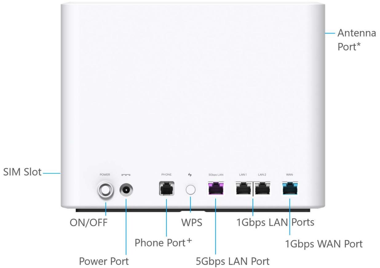
\*For external 3.4-5GHz antenna supporting high sub-6 bands
