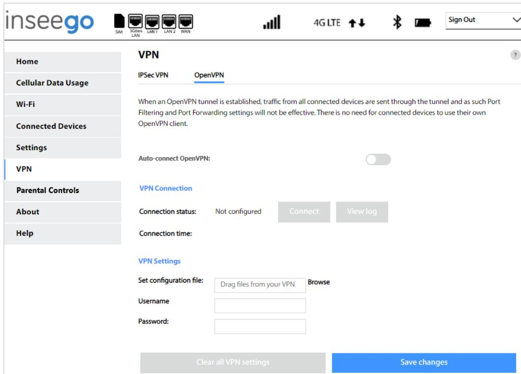
**NOTE:** When an OpenVPN connection is established, Port Filtering and Port Forwarding settings are not effective, as traffic from all connected devices goes through the OpenVPN tunnel.
