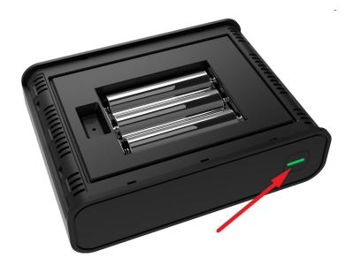
The LED indicator is green when the device is turned on.
