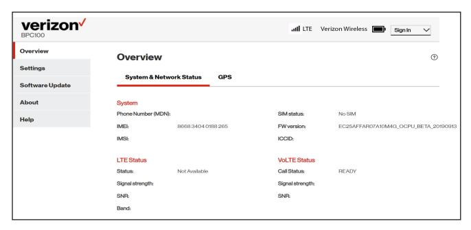
Select the **GPS** tab to display GPS coordinates of the current location of the BPC100. Latitude, longitude, altitude, and accuracy are shown as defined by GPS NMEA strings.
