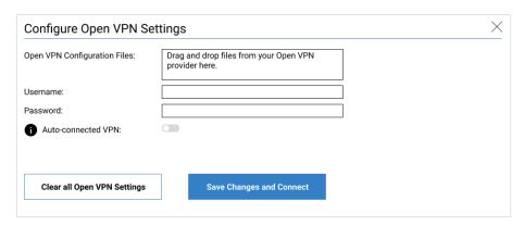
**Open VPN Configuration Files:** Drag and drop the Open VPN configuration files from your Open VPN provider in the file upload area.
