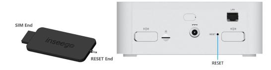
2. Press the SIM tool on the button for about five to six seconds, then your 5G indoor router will restart.
